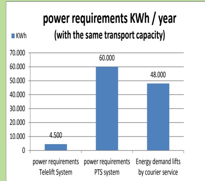
The energy requirement of a Telelift system represents one tenth of the energy requirements of a pneumatic tube system. The message service performed by pneumatic tube systems additionally requires 10 times the energy of an alternative Telelift system.
