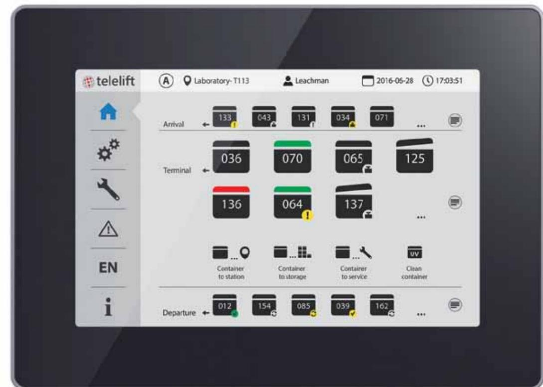
Operation of the Telelift system is easy and self-explanatory. The new terminal has 6 main entry areas for users: home, settings, service, error messages, language setting and operating manual:
